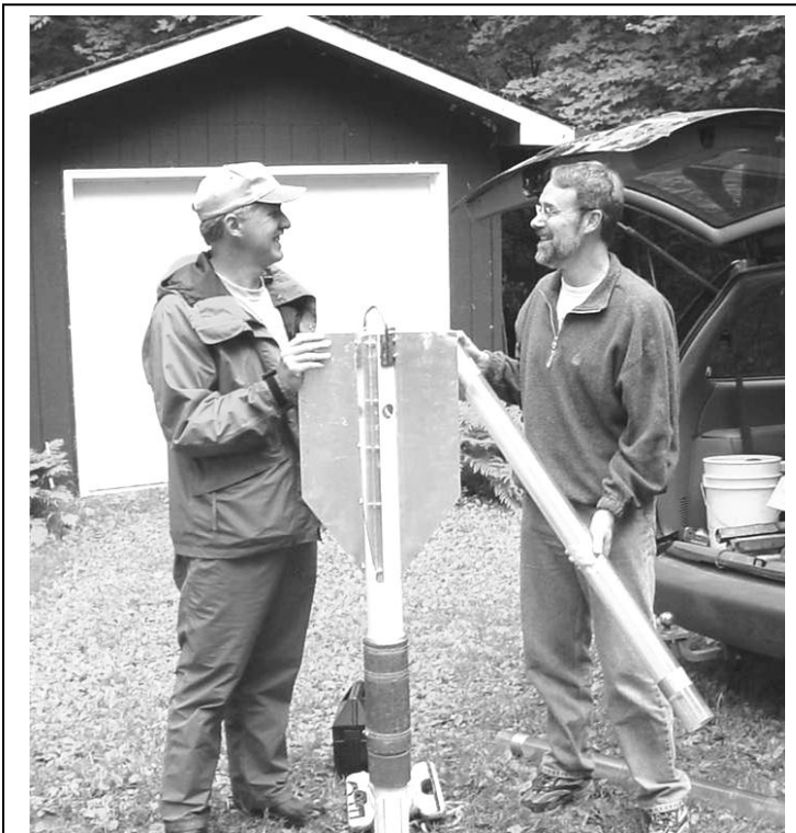
Paleolimnologist Paul Garrison and Blue Lake resident Mark Bergeon preparing to use “the bomb”, the piece of equipment with which they will retrieve the core sample from the bottom of Blue Lake.
